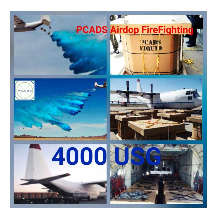
at a chosen altitude, so an aircraft can fly over a wildfire at a safe height, like 5,000' AGL (above ground level), when it performs a drop. The aircraft simply tips the nose up over the target and the PCADS units roll out the back, which is much safer and easier to do than having to dive down close to the ground, maneuvering through canyons, like most air-tankers do.
