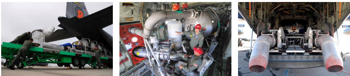
Fig. 2: Modular Airborne Fire Fighting System (MAFFSII).
