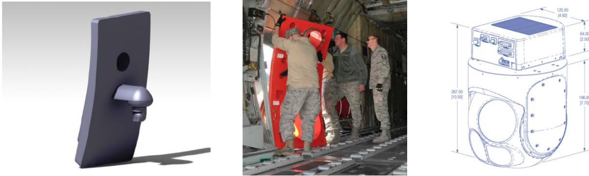
Fig. 7: Modular paratrooper door for FLIR installation.
